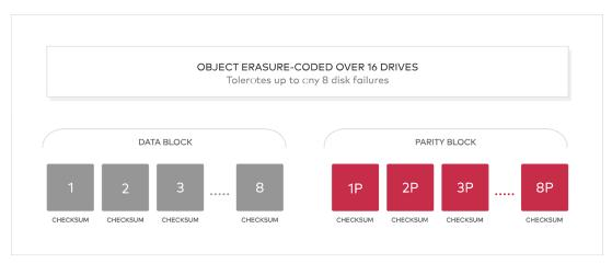
Figure 5: MinIO's data protection schemes cover failure and silent data corruption.
